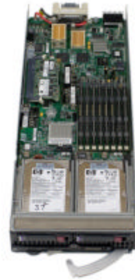
Figure 1: HP blade server
