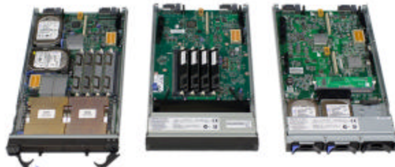
Figure 2: IBM blade server, plus memory and I/O expansion blades
